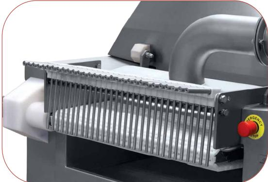
unique removal system of brine overflow from surface of raw material
