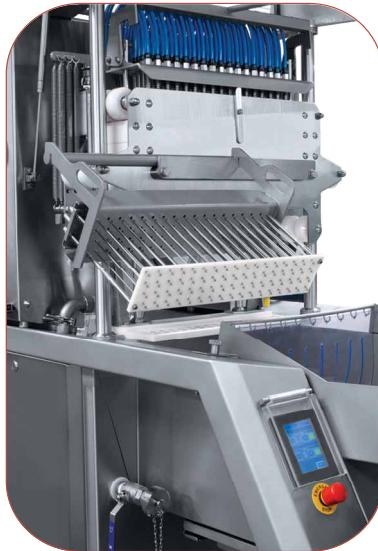
quick replacing needle head
