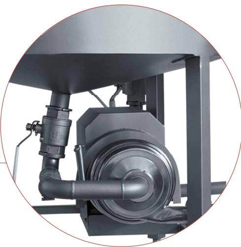
An efficient **centrifugal pump**, forcing the brine circulation, enables excellent blending of dry ingredients in water.
